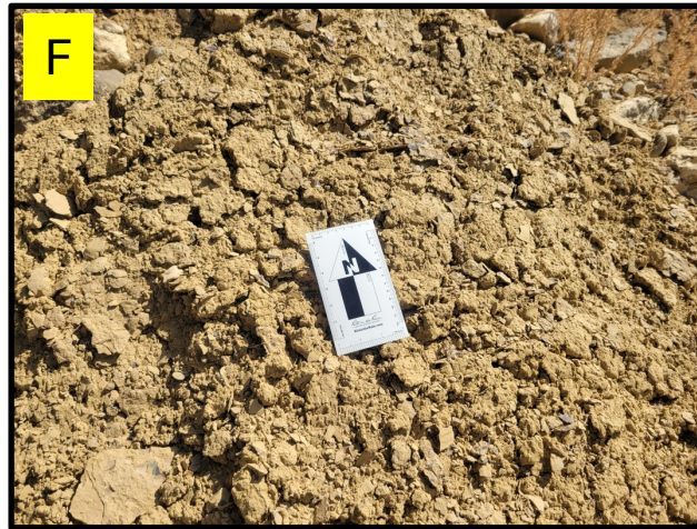
Figure F. Weathered Mancos Fm ( Q_{wm} ) is highly friable, light brown color, but still produces some shallow marine fossils. The brown color indicative of clay weathering.
